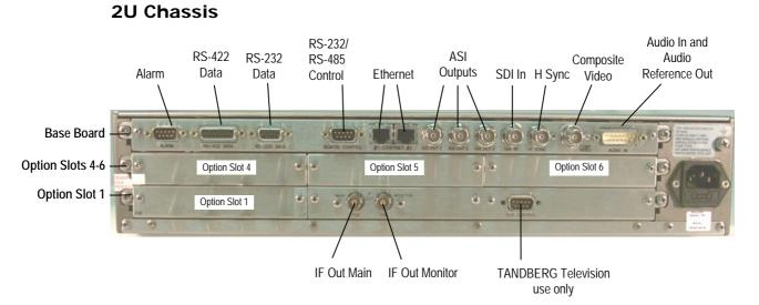
Figure 1.12: E5740 (2U) Rear Panel Component Parts and Connectors
